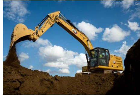
Cat's 320 electric excavator
